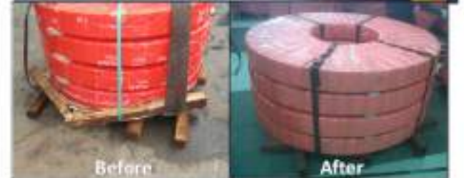
Steel coil packing – Wood eliminated
