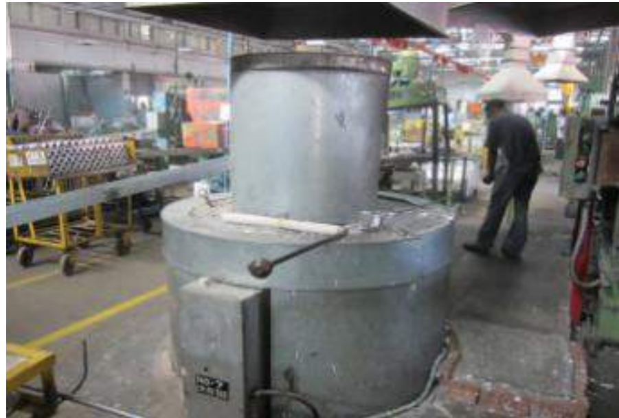
Electrical Fired AL melting Furnace
